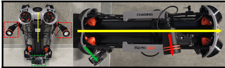
Fig. 1: The underwater ROV captured from two different angles. The position and orientation of the camera and light sources are highlighted by green and red markings, respectively. The yellow arrows indicate the forward orientation of the drone.
